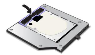
6. Insert the ThinkPad Serial Hard Drive Bay Adapter III into the Serial Ultrabay Enhanced bay.
